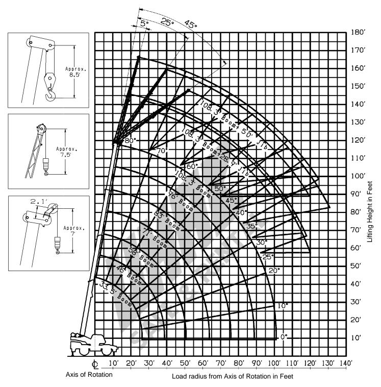
**NOTE:** Boom and jib geometry shown are for unloaded condition and machine standing level on firm supporting surface. Boom deflection and subsequent radius and boom angle change must be accounted for when applying load to hook.
