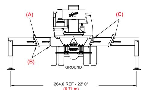
(A) Pins must be disengaged for this outrigger configuration
