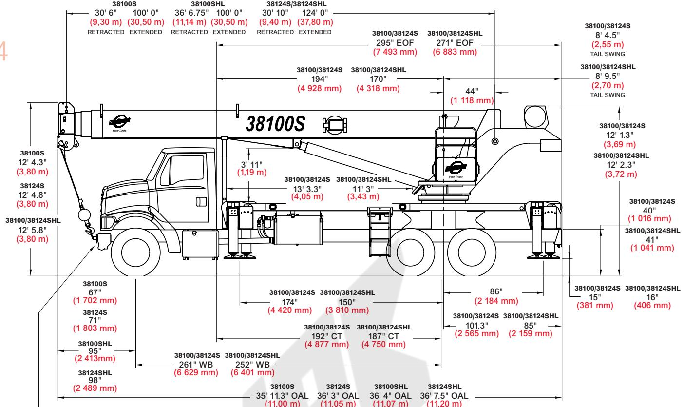
A front center stabilizer is required on installations equipped with the short sub frame (38100SHL & 38124SHL)
