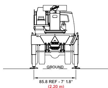
NOTE: Lifting personnel with crane in this outrigger configuration is strictly prohibited. Use only fully extended outrigger configuration when lifting personnel.
