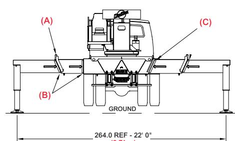
(A) Pins must be disengaged for this outrigger configuration
