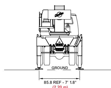
**NOTE:** Lifting personnel with crane in this outrigger configuration is strictly prohibited. Use only fully extended outrigger configuration when lifting personnel.
