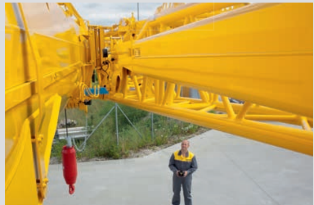
Hydraulic assistance for assembly of the swing-away jib with BTT
