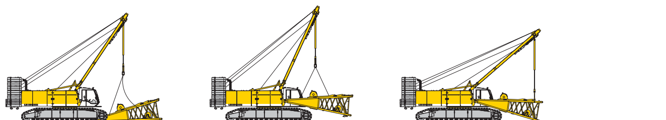
Unloading and assembly of boom foot
