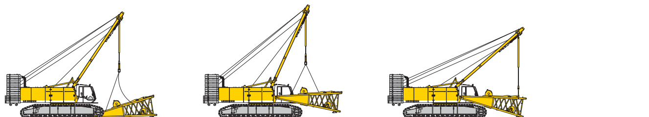
Unloading and assembly of boom foot
