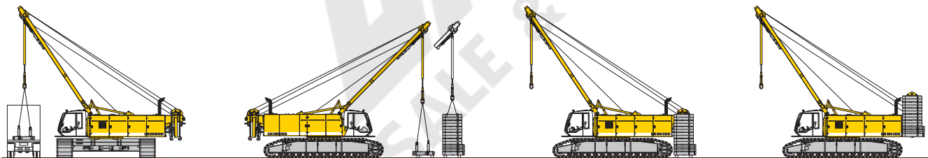
Unloading and assembly of counterweight
