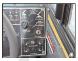
Optional rated capacity limiter--four position operator selection "lifting condition" that constantly monitors actual lifting conditions
