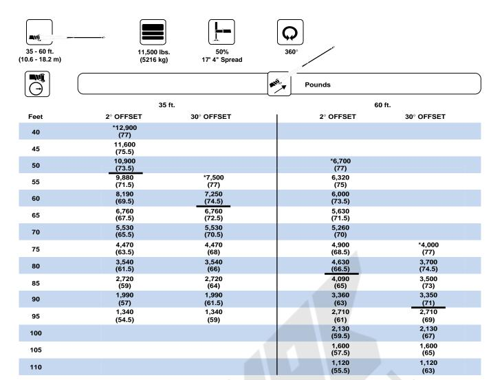
\*This capacity is based upon maximum boom angle.
