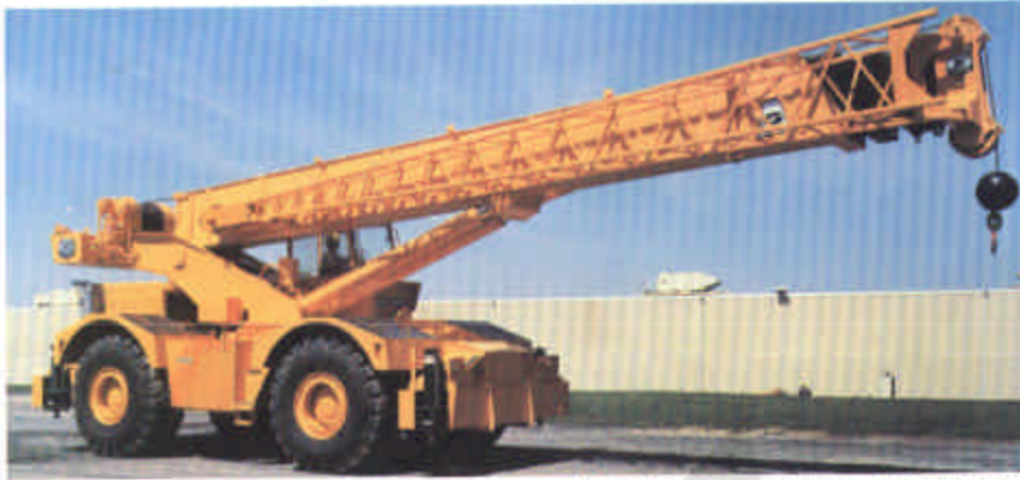
The "Swing Away" lattice boom extension stows laterally along side the boom base section and swings easily into working position to provide 121' (36.9m) tip height with the standard boom and 147' (44.8m) tip height with the optional boom.
