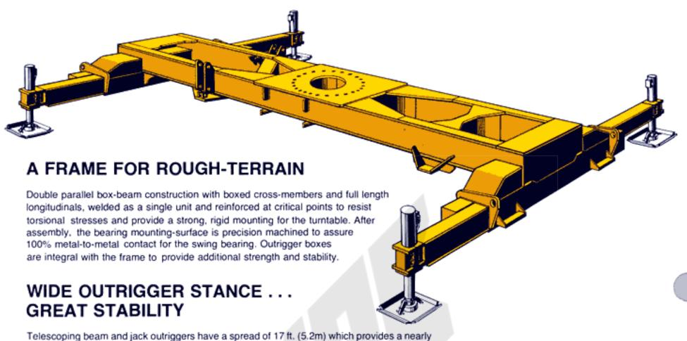
square stance for outstanding stability throughout the 360° lifting range. Jacks have a vertical stroke of 21 in. (533mm) and are equipped with integral holding valves. The exclusive Grove Spin-lock†, which permits the jack to be locked mechanically in any position, is available as optional equipment.
