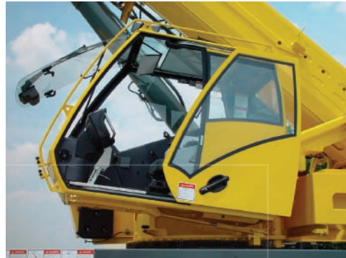
SUPERSTRUCTURE CAB Hydraulically offsets to 20°; all aluminum construction
