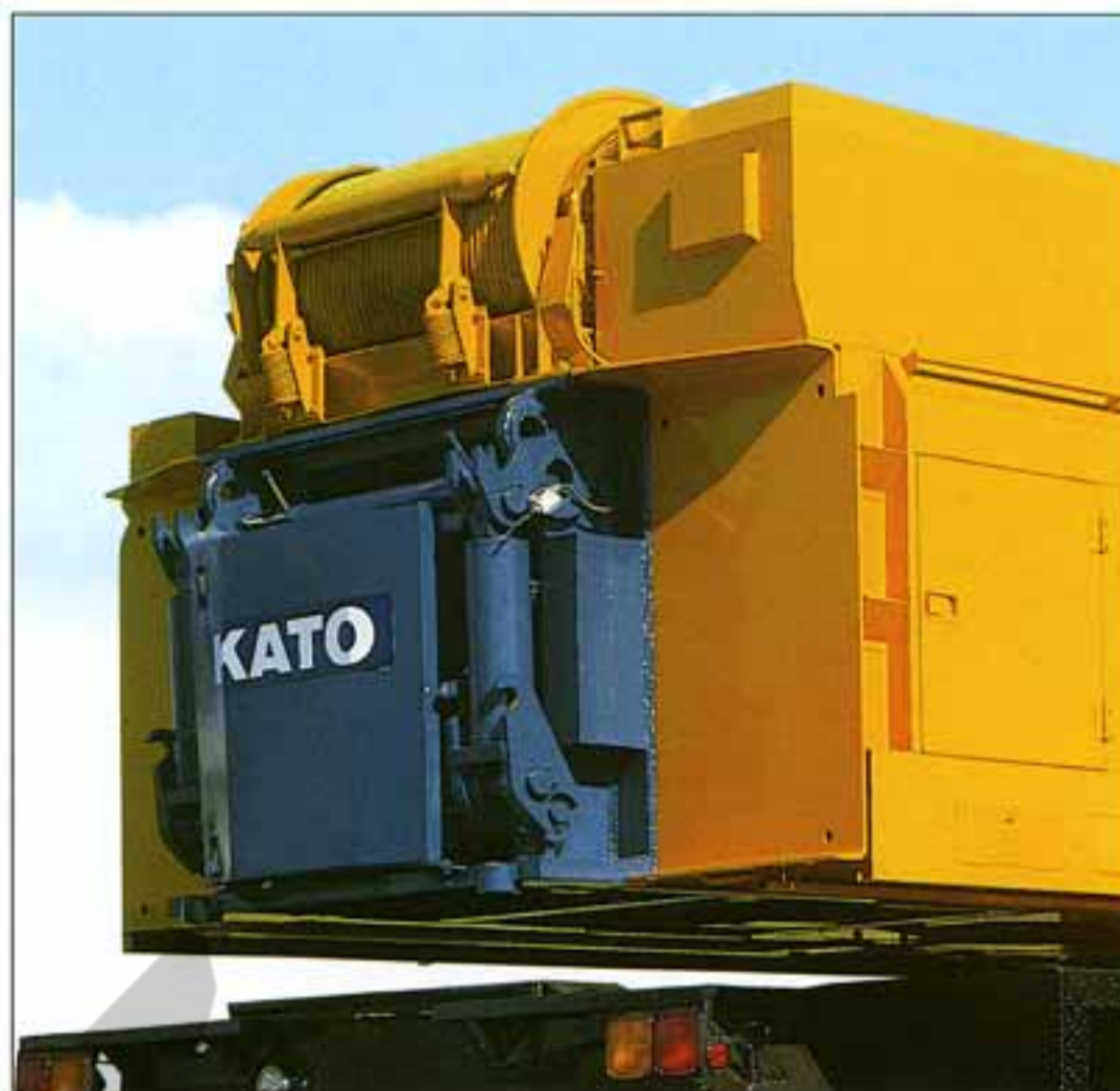
Linkage-type counterweight removal device
