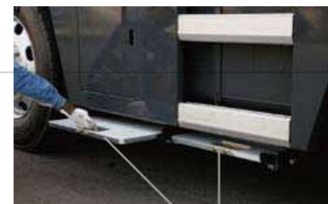
Aluminium step as standard equipment (600×600mm)
