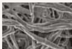
Conventional filter (paper fiber)
