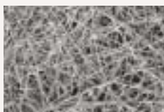
Super fine filter (glass fiber)
